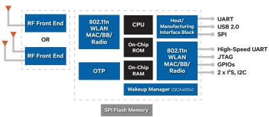
The QCA4002/4004 are an intelligent platform for the Internet of Everything. The complete networking platform enables customers to add full-featured Wi-Fi to a wide variety of products with minimal development effort and cost. It supports a network stack along with SSL security, enabling full-featured internet connectivity and reliable information exchange in a small, low-cost system.
